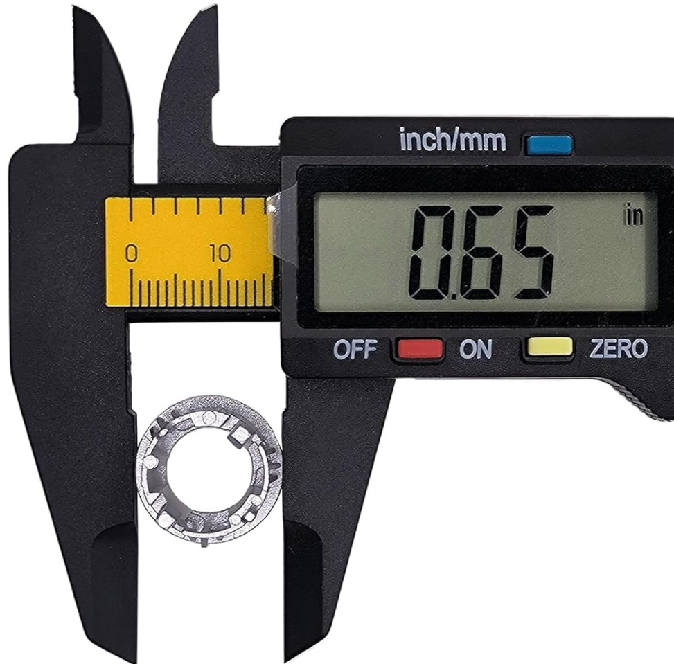
Figure 5.1: Measurement of the button holder, indicating a diameter of 0.65 inches.
