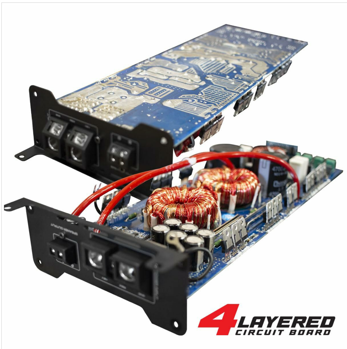
Figure 3: Internal view of the DB Drive WDX2000.1 mini amplifier, highlighting the advanced 4-layered circuit board design and robust internal components, including large toroidal transformers.
