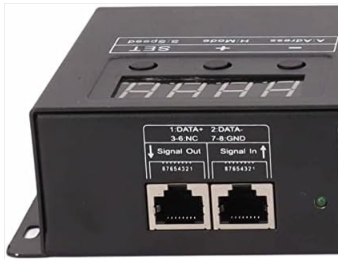
Figure 4.2: Close-up view of the DMX Signal In and Signal Out RJ45 interfaces.
