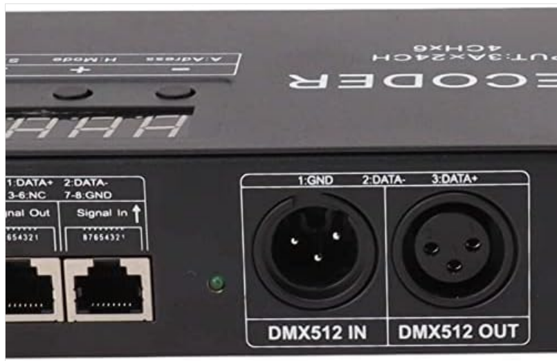
Figure 4.1: Close-up view of the DMX512 IN and DMX512 OUT XLR 3-pin connectors.
