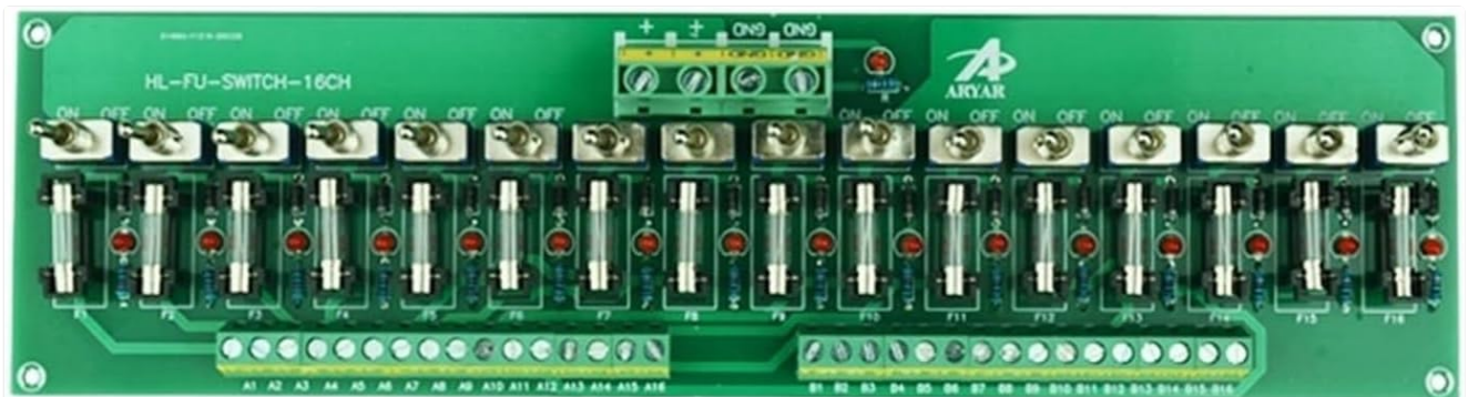
Figure 4.3: An angled view of the module, providing a clearer look at the individual switches and the transparent fuse holders for each of the 16 channels. The "ON" and "OFF" markings for the switches are visible.
