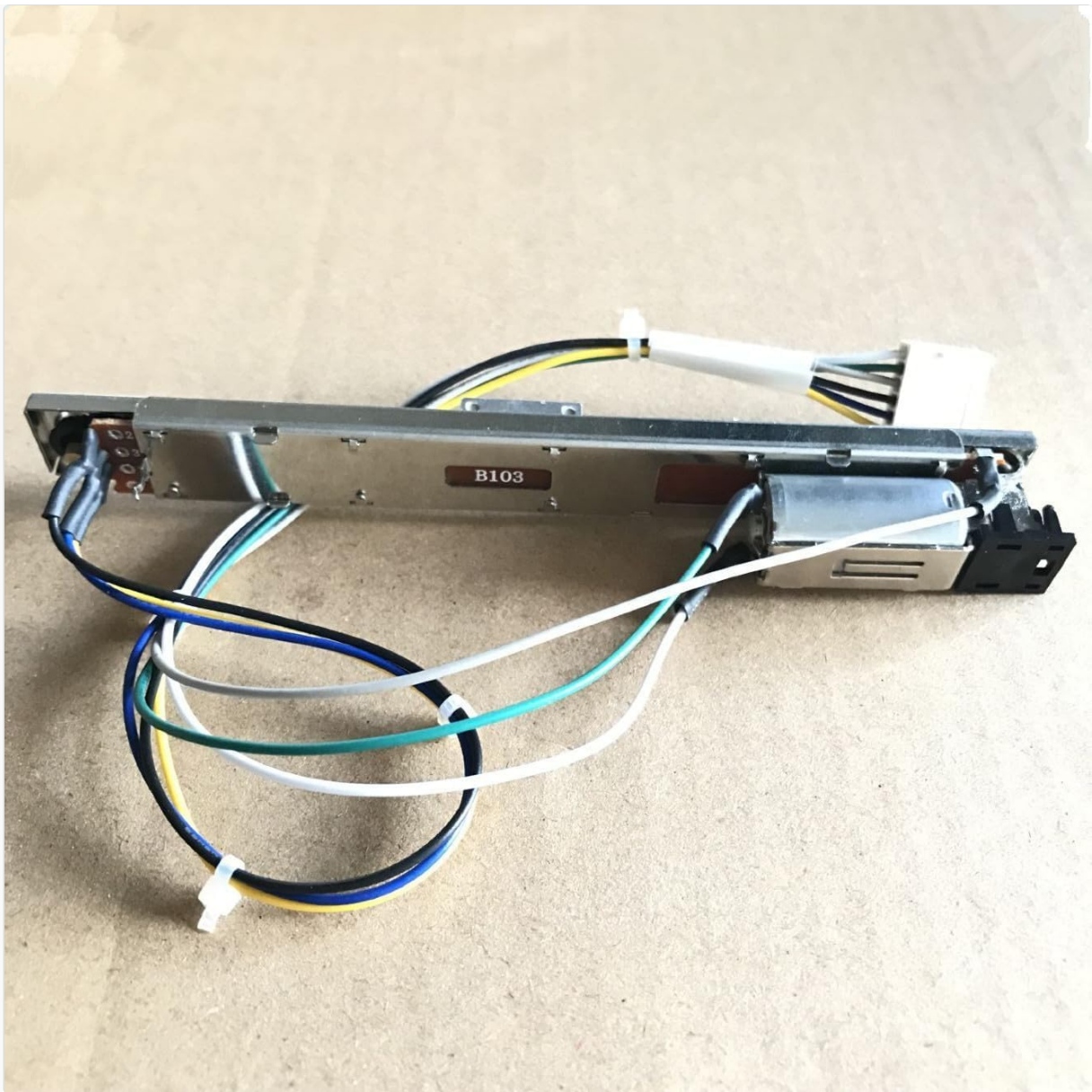
Image: A detailed view of a single motorized fader, highlighting its robust construction and integrated motor mechanism.
