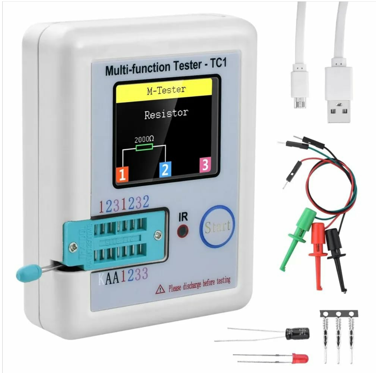
Image: The LCR-TC1 tester showing a resistor being measured, with the resistance value displayed on the screen.
