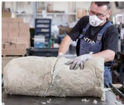
Figure 3: The Maestro 40 features rock wool insulation for efficient heat retention and a safe-to-touch exterior.
