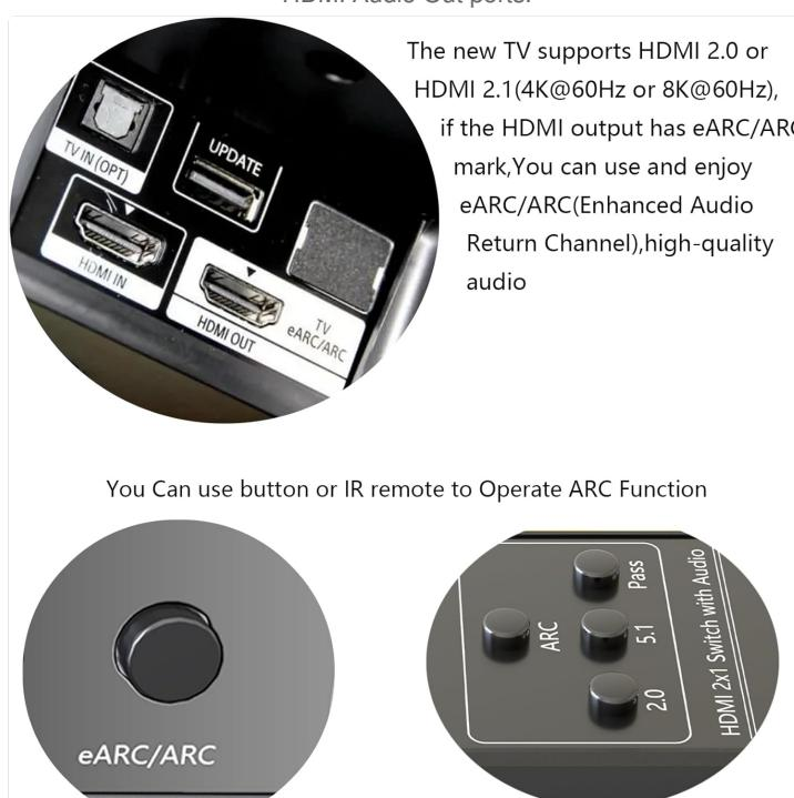
The eARC/ARC function can be activated or deactivated using the dedicated 'eARC/ARC' button on the device's front panel or the 'ARC' button on the IR remote control. This allows for audio return channel functionality with compatible televisions.
