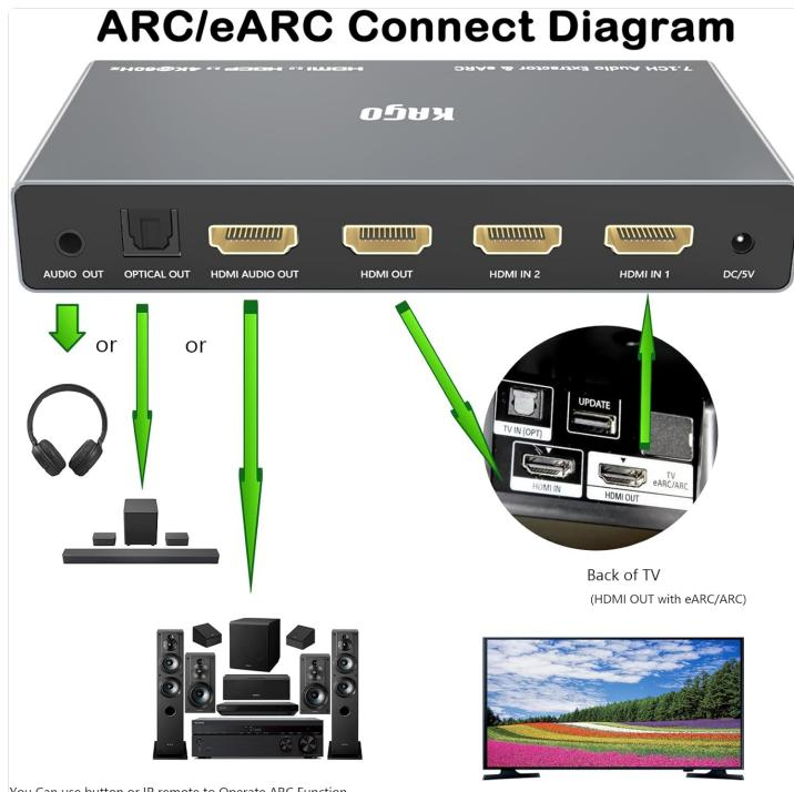
For ARC/eARC functionality, connect the HDMI-ARC/eARC output port of your television to the HDMI IN 1 port of the KAGO HDMI Audio Extractor Splitter. Audio can then be extracted to headphones, a soundbar, or a home theater system via the Audio Out, Optical Out, or HDMI Audio Out ports.
