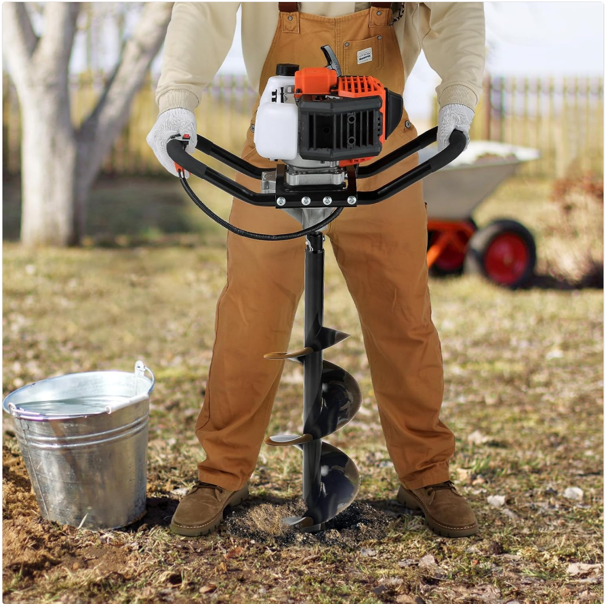
Figure 6: Proper operating stance for drilling.
