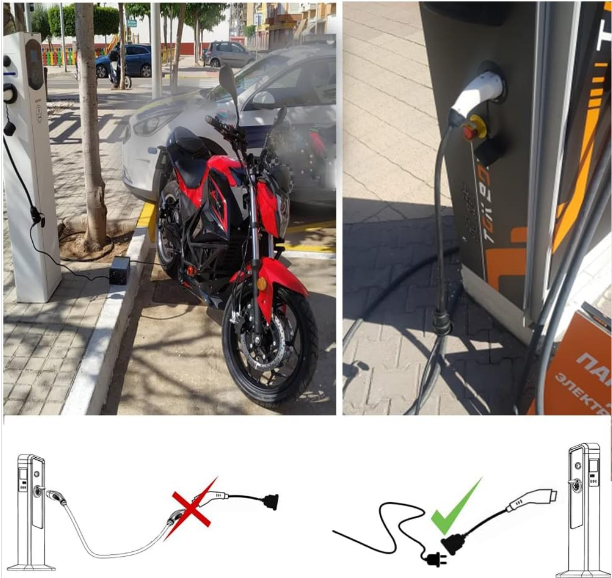
Figure 5.3: Examples of the adapter in use for EV charging. The image shows both correct and incorrect connection methods, emphasizing the proper way to connect the adapter for charging.
