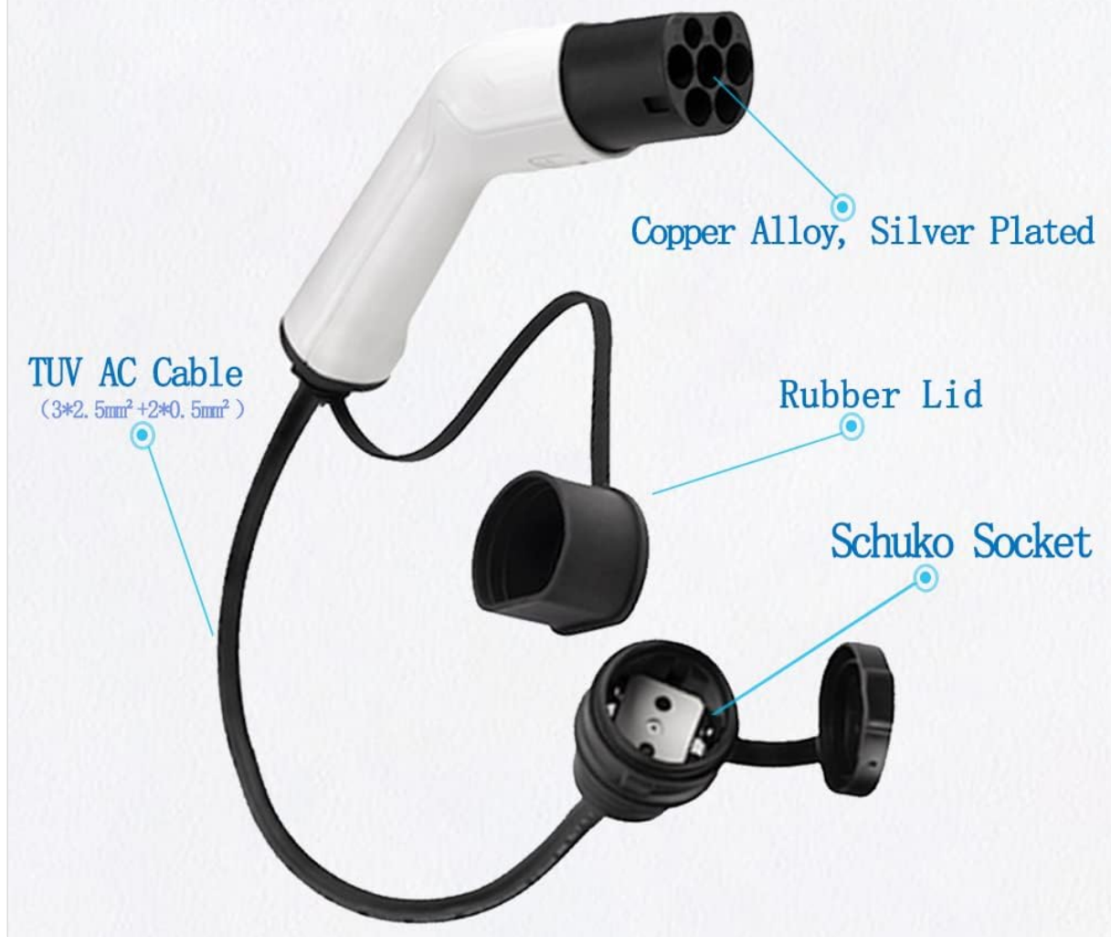
Figure 3.3: Detailed view of the Type 2 plug and Schuko socket, showing internal components. The image points out the copper alloy, silver-plated contact pins, the rubber lid for protection, and the TUV AC cable specifications (3*2.5mm 2 + 2*0.5mm 2 ).
