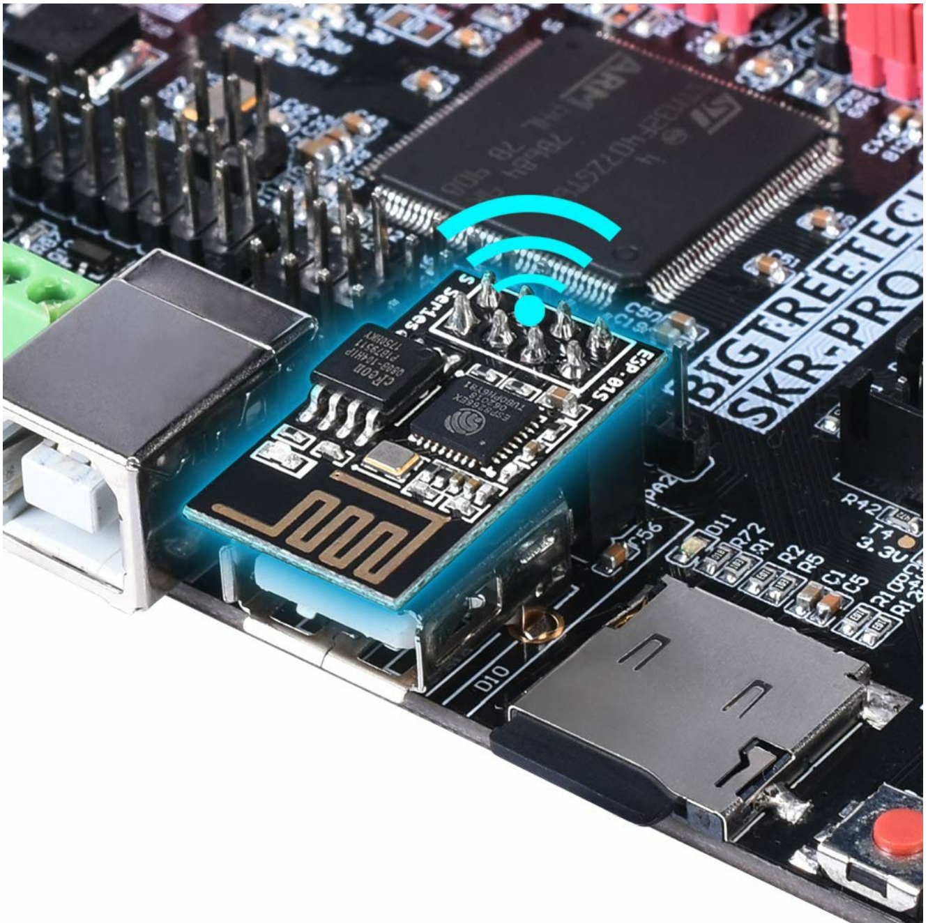
Image: A close-up view of the WIFI module slot on the SKR Pro V1.2 board, showing a module installed and indicating its wireless communication capability.
