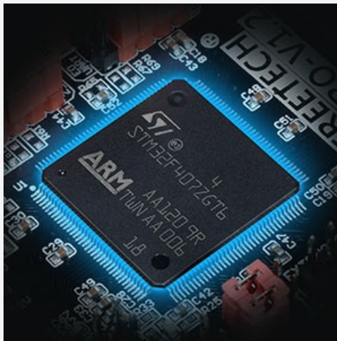
Image: A close-up of the STM32F407ZGT6 microcontroller chip, the core of the SKR Pro V1.2 board, responsible for processing and executing firmware commands.
