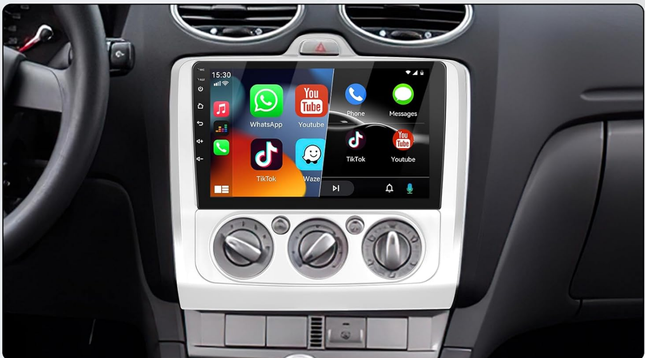
Figure 5.1: Display of Apple Carplay and Android Auto interfaces, highlighting the ability to access phone applications and features on the car radio.
