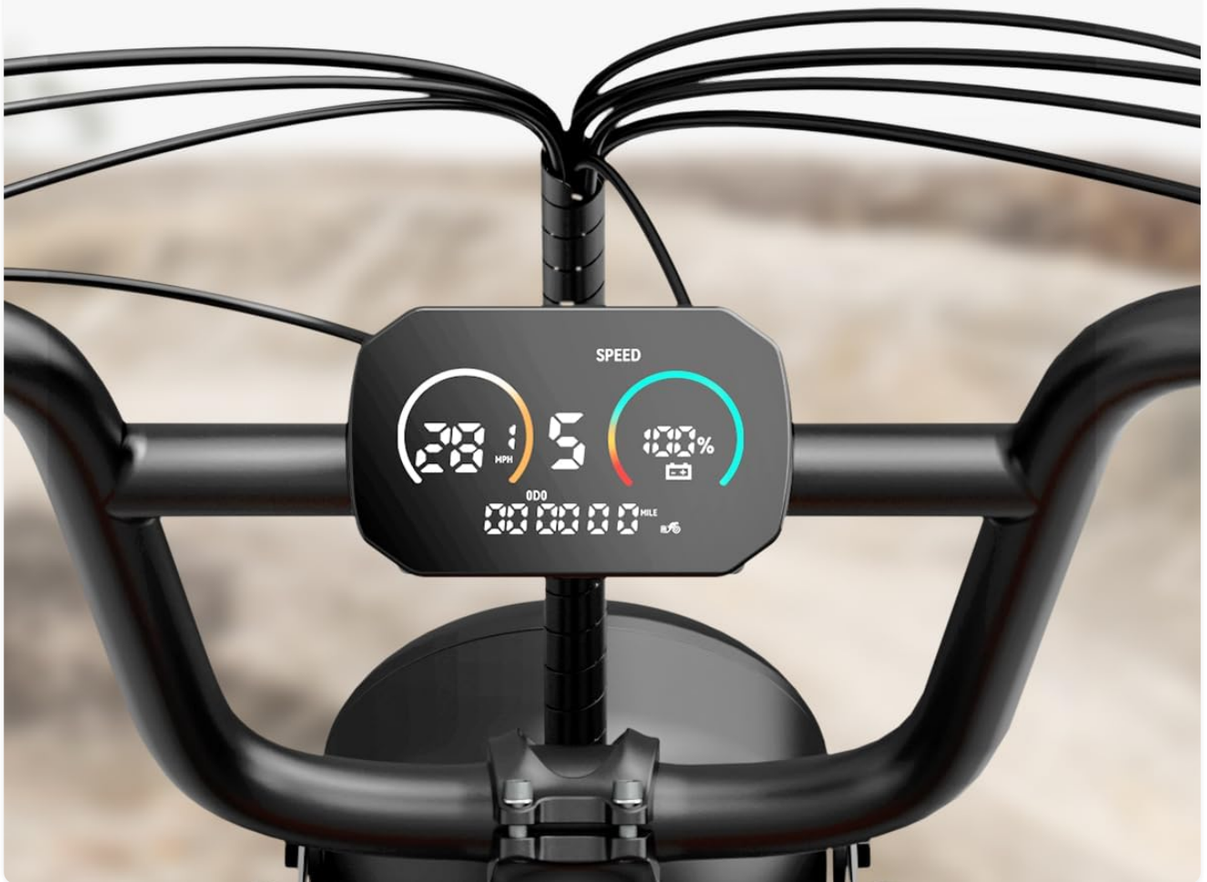
Figure 3.10: The intelligent LCD display system, providing comprehensive ride data.
