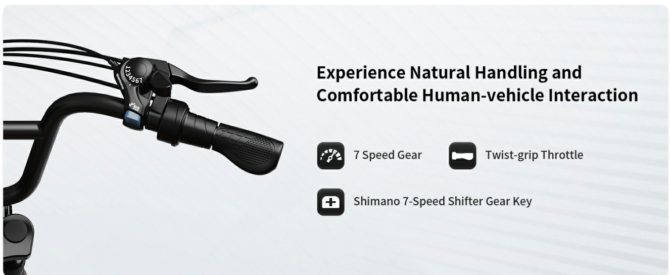
Figure 3.13: Close-up of the 7-speed gear shifter and twist-grip throttle.
