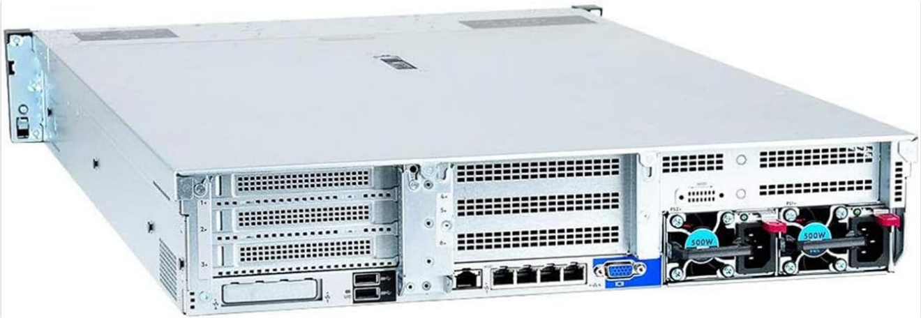
Figure 4.4: Rear view of the HPE ProLiant DL380 Gen10 server, showing the redundant power supply units and network ports.
