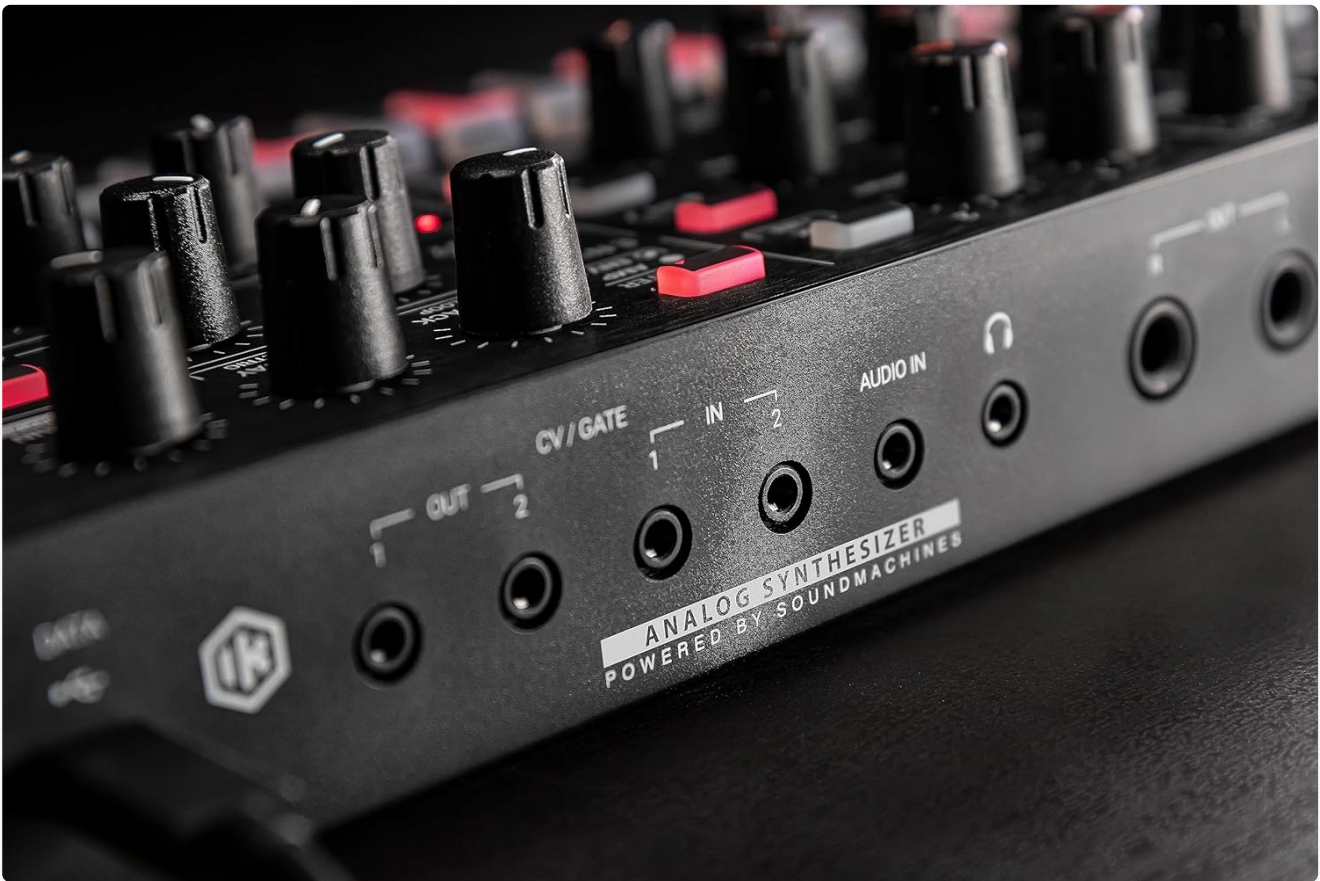
Figure 3.1: Rear panel connections including USB, CV/GATE, Audio In/Out, and Headphones.
