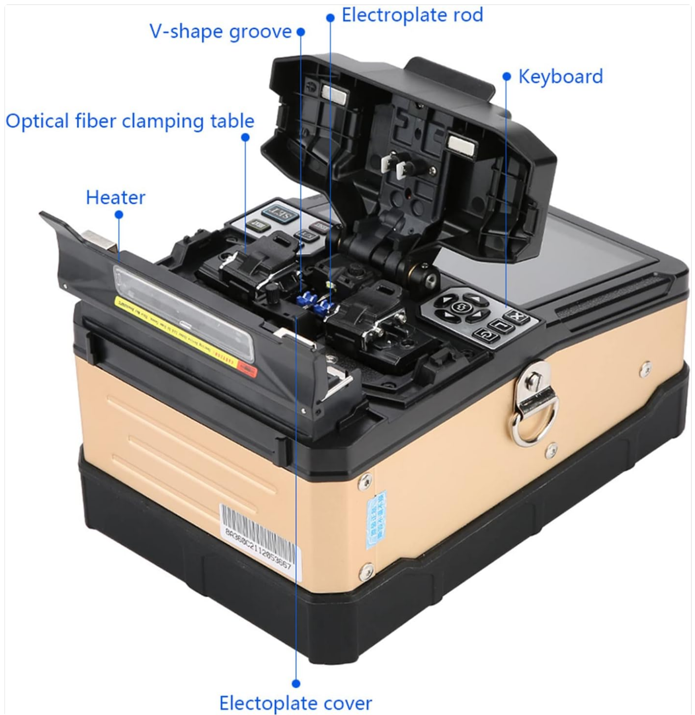
Figure 2.1: Internal Components of the FS-60C Fusion Splicer
