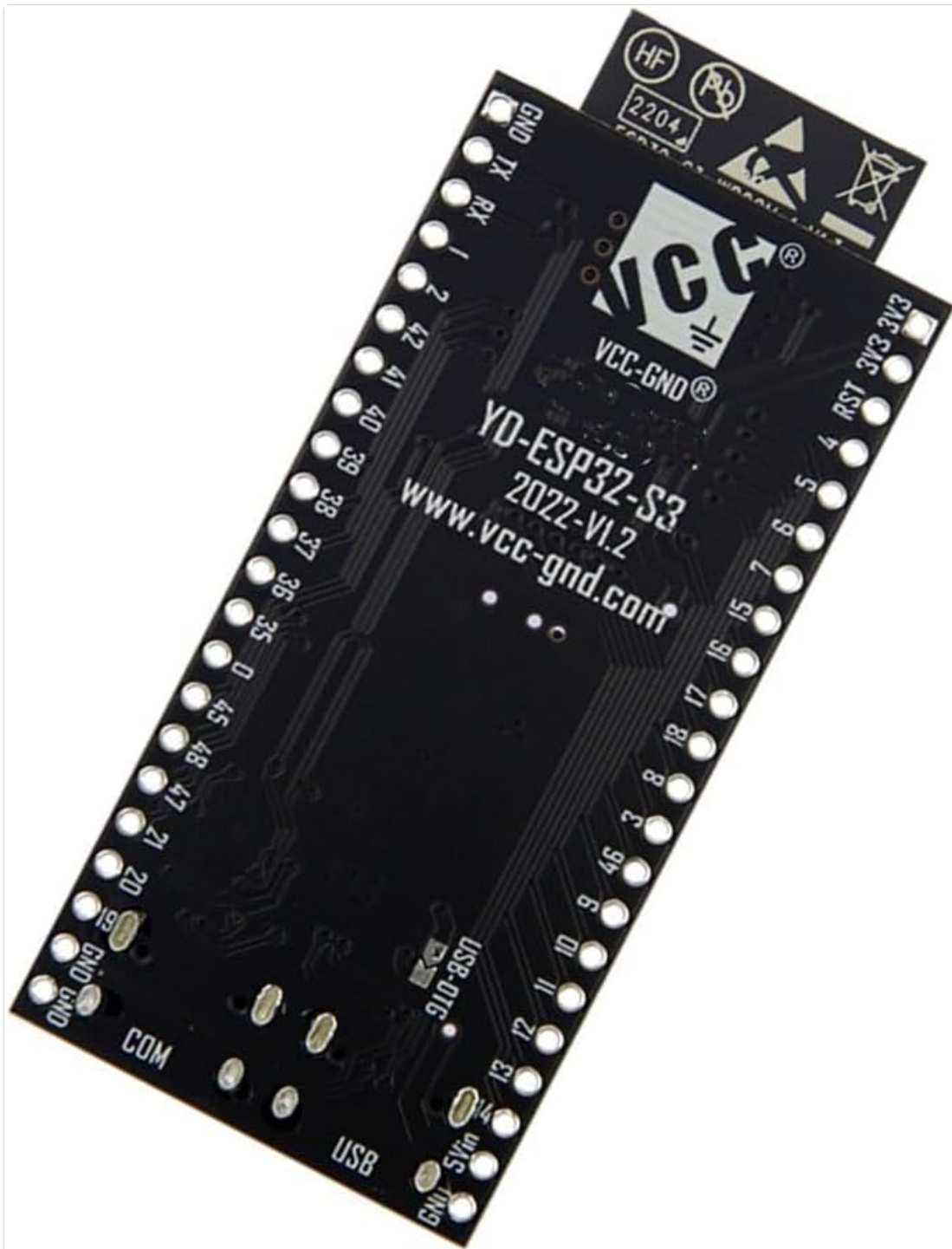
Figure 4.3: Back View of the ESP32-S3 Core Board N8R8
