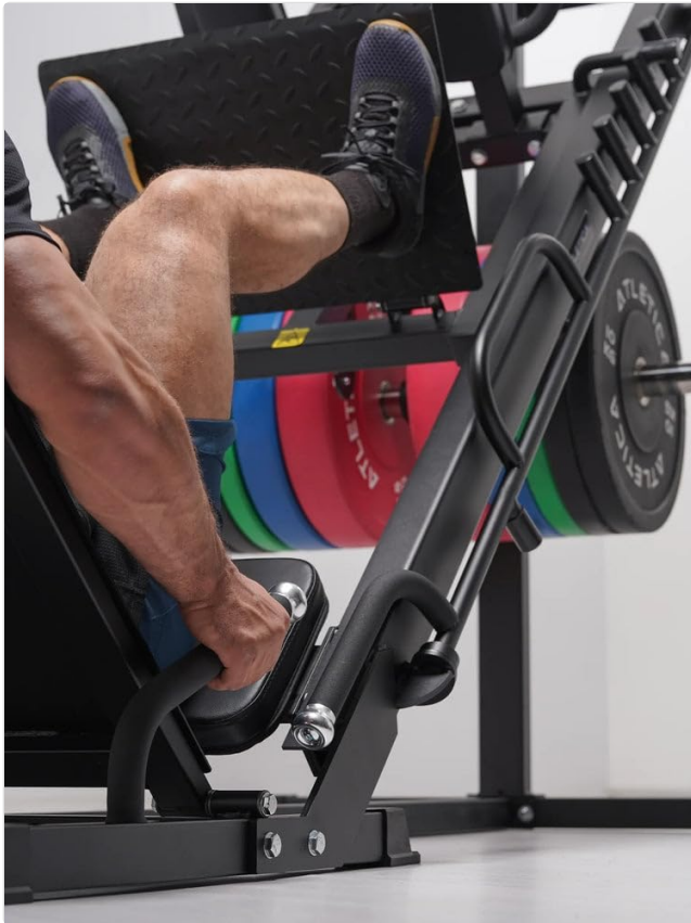
Image: Detail of the footplate and safety handles. These handles are used to engage and disengage the safety catches.
