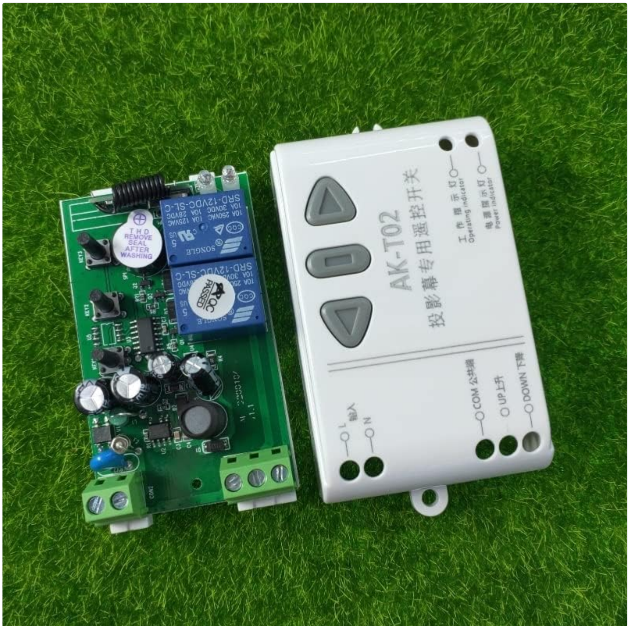
Image 5.1: An internal view of the AK-T02 receiver module, showing the circuit board with relays and wiring terminals. This image provides context for understanding the connection points for power input and motor output.
