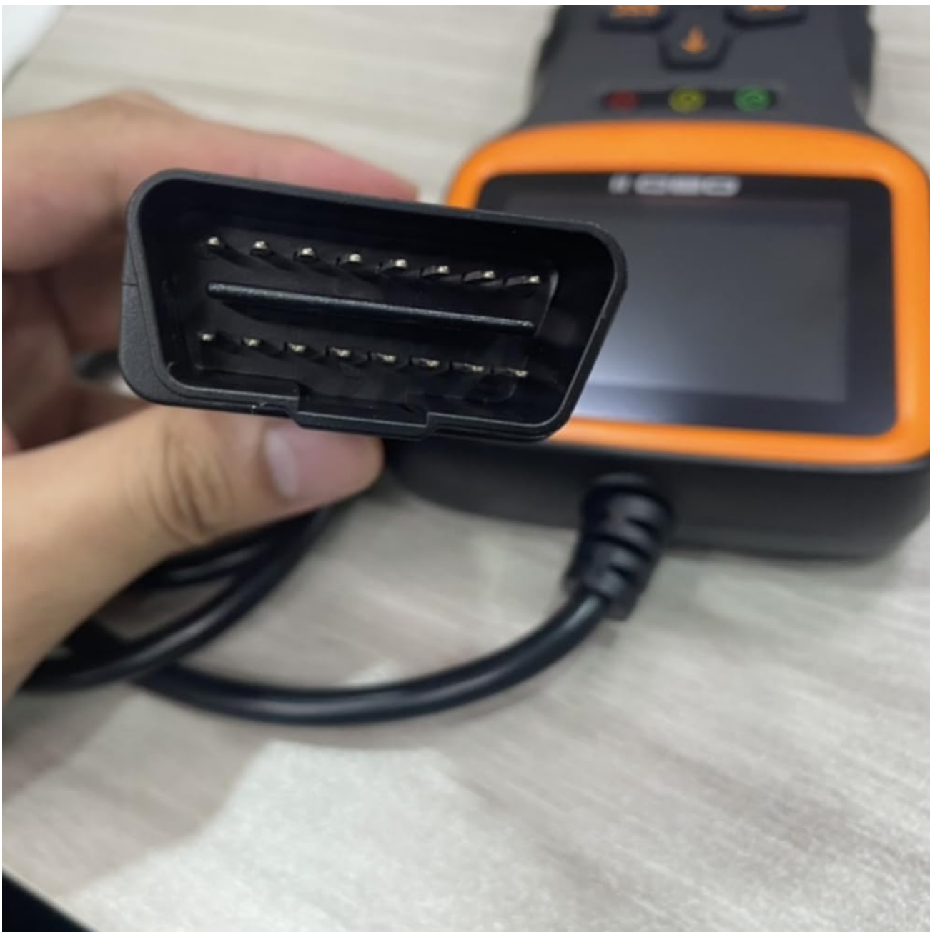
Figure 5: Close-up view of the V317's OBD2 connector, which plugs into the vehicle's diagnostic port.
