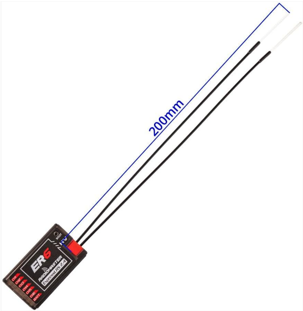
Image 2.3: The ER6 receiver with its 200mm dual antennas connected, illustrating proper antenna length.
