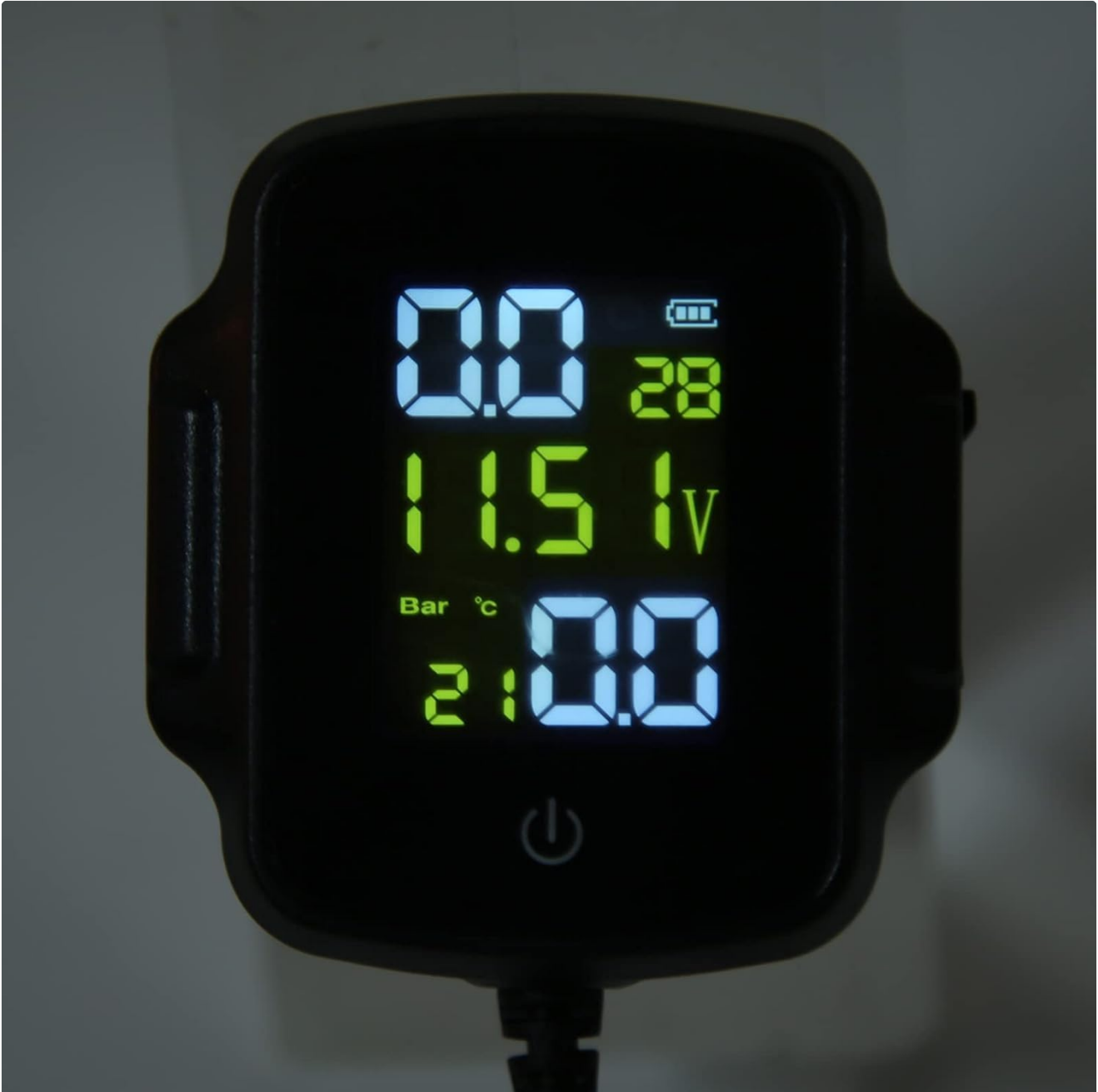
Image: A detailed view of the TPMS display, clearly showing the digital readouts for tire pressure (top), battery voltage (middle), and tire temperature (bottom), along with a battery level indicator.
