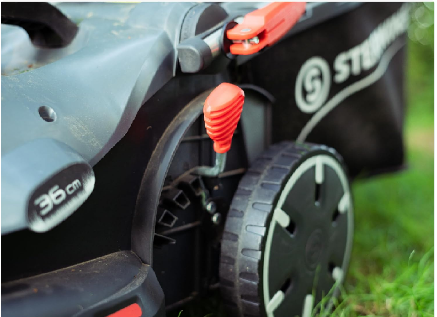
Image 4: Close-up of the cutting height adjustment lever.
