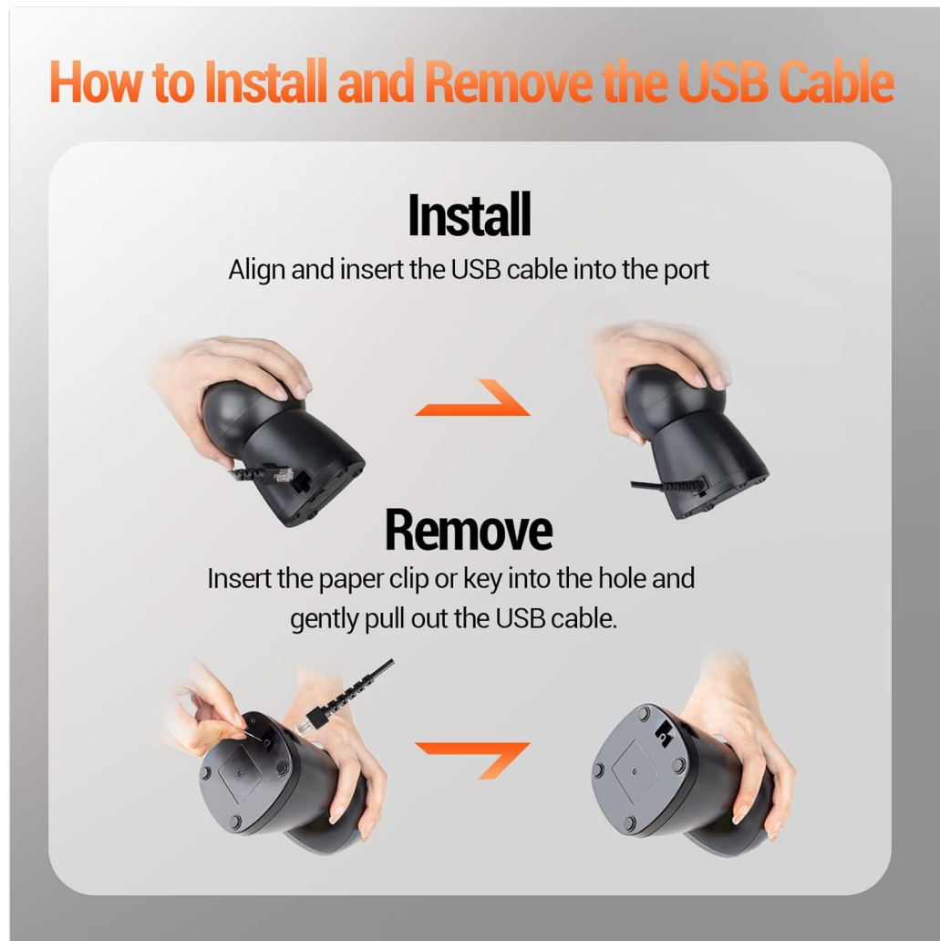
Image 3.3: USB Cable Installation and Removal. This image provides a visual guide for inserting the USB cable into the scanner's port and for safely removing it using a paper clip or key in the designated pinhole.
