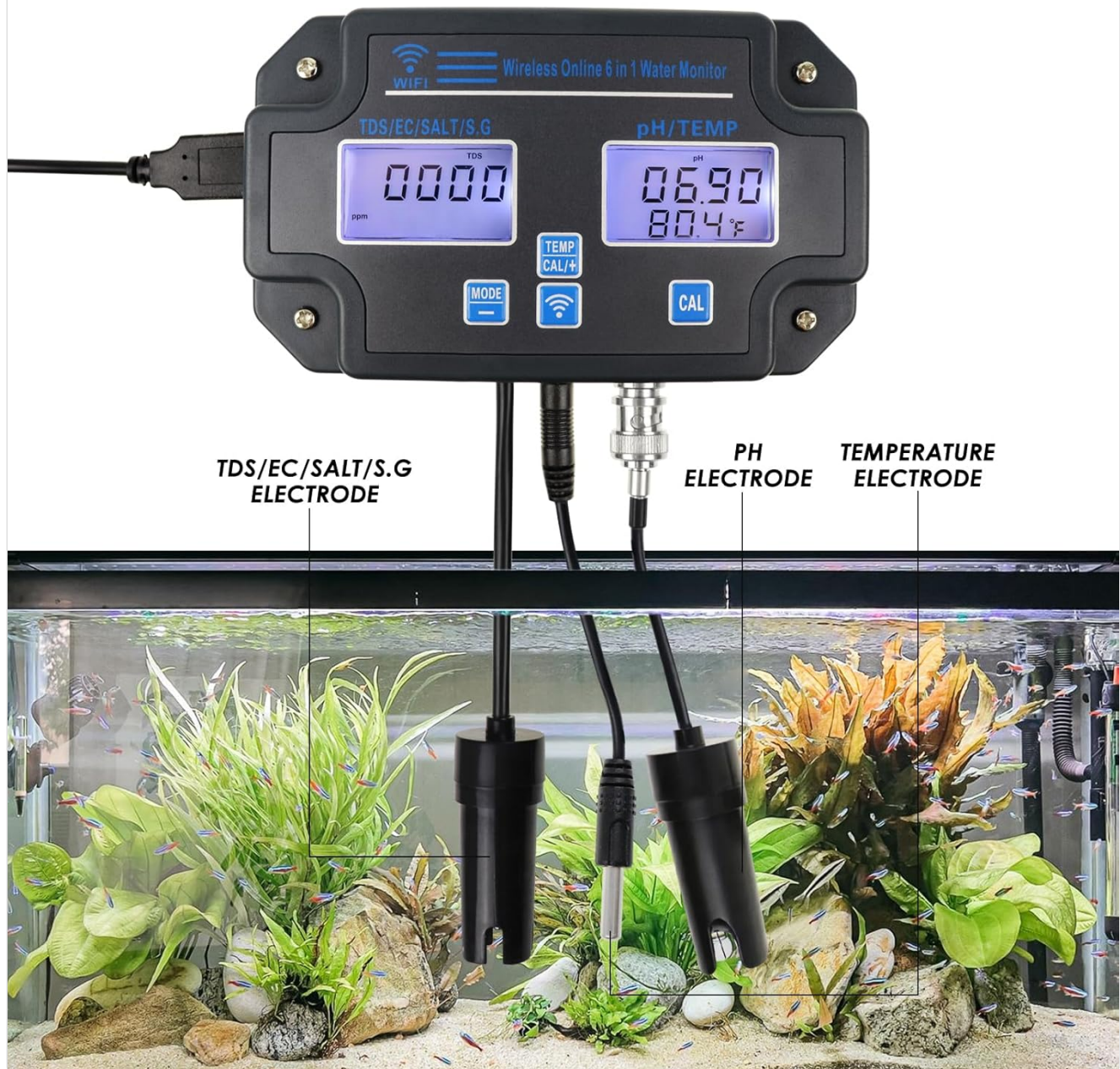
Image: The meter actively monitoring water parameters in an aquarium setup.
