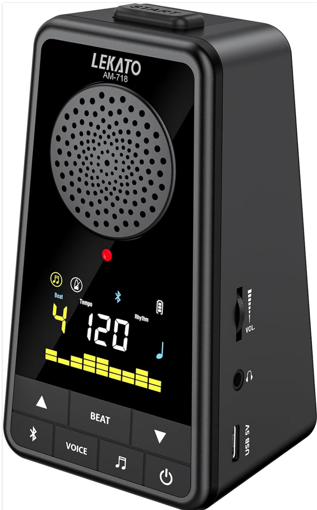
Image: Front and side view of the LEKATO AM-718 metronome, highlighting its speaker, display, and control buttons.
