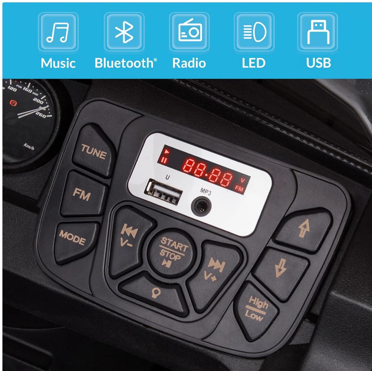
Image: A close-up view of the Kidzone ride-on truck's control panel, detailing the buttons for music, Bluetooth connectivity, radio, LED light control, and a USB port for media playback.
