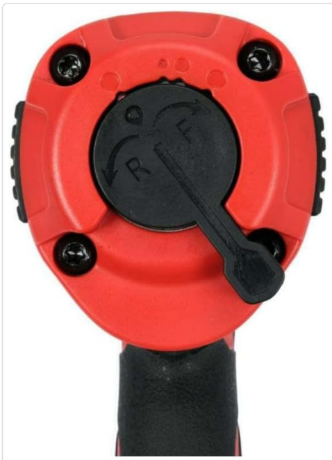
Figure 3.2: Direction Control Switch. Located at the rear of the tool, this switch allows selection between forward (tightening) and reverse (loosening) rotation. The 'R' indicates reverse, and 'F' indicates forward.
