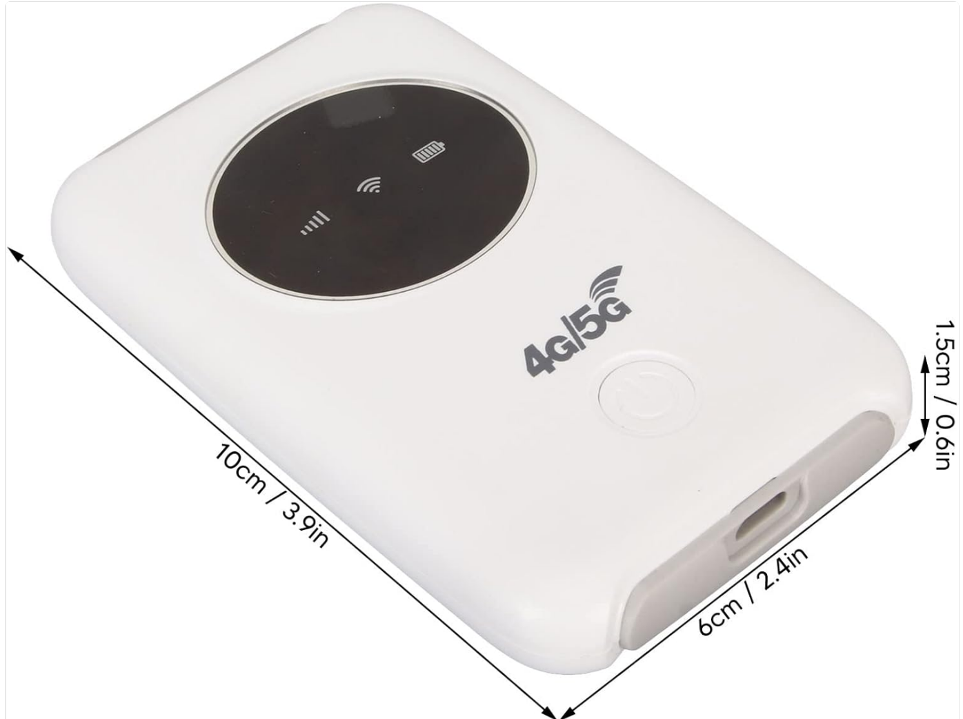
Image: The ASHATA mobile hotspot with its approximate dimensions (10cm/3.9in length, 6cm/2.4in width, 1.5cm/0.6in height) overlaid, illustrating its compact size.
