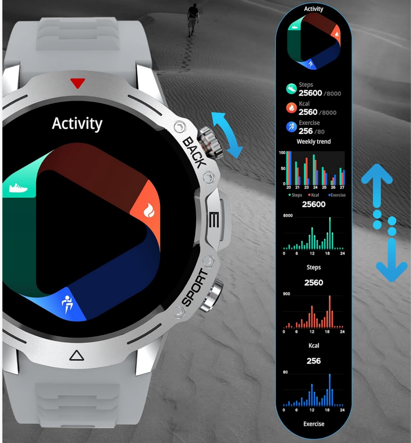
Image: Visual guide demonstrating the use of the digital crown for scrolling on the G102 Smart Watch.
