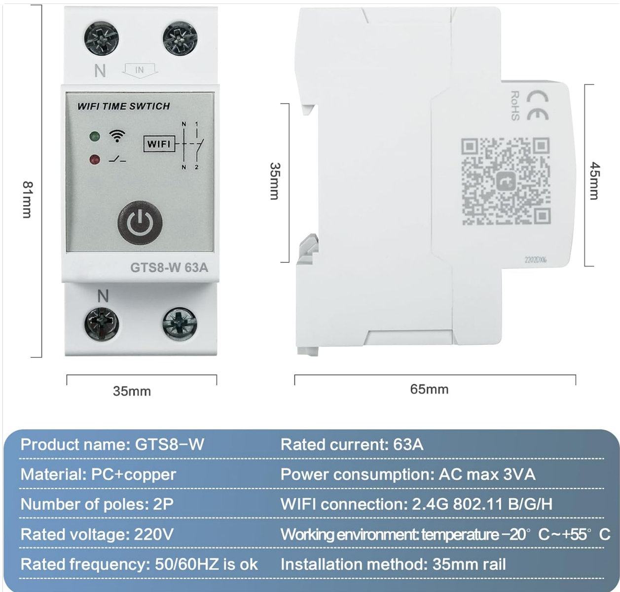
Image 4.1: Detailed dimensions and key specifications of the GTS8-W.
