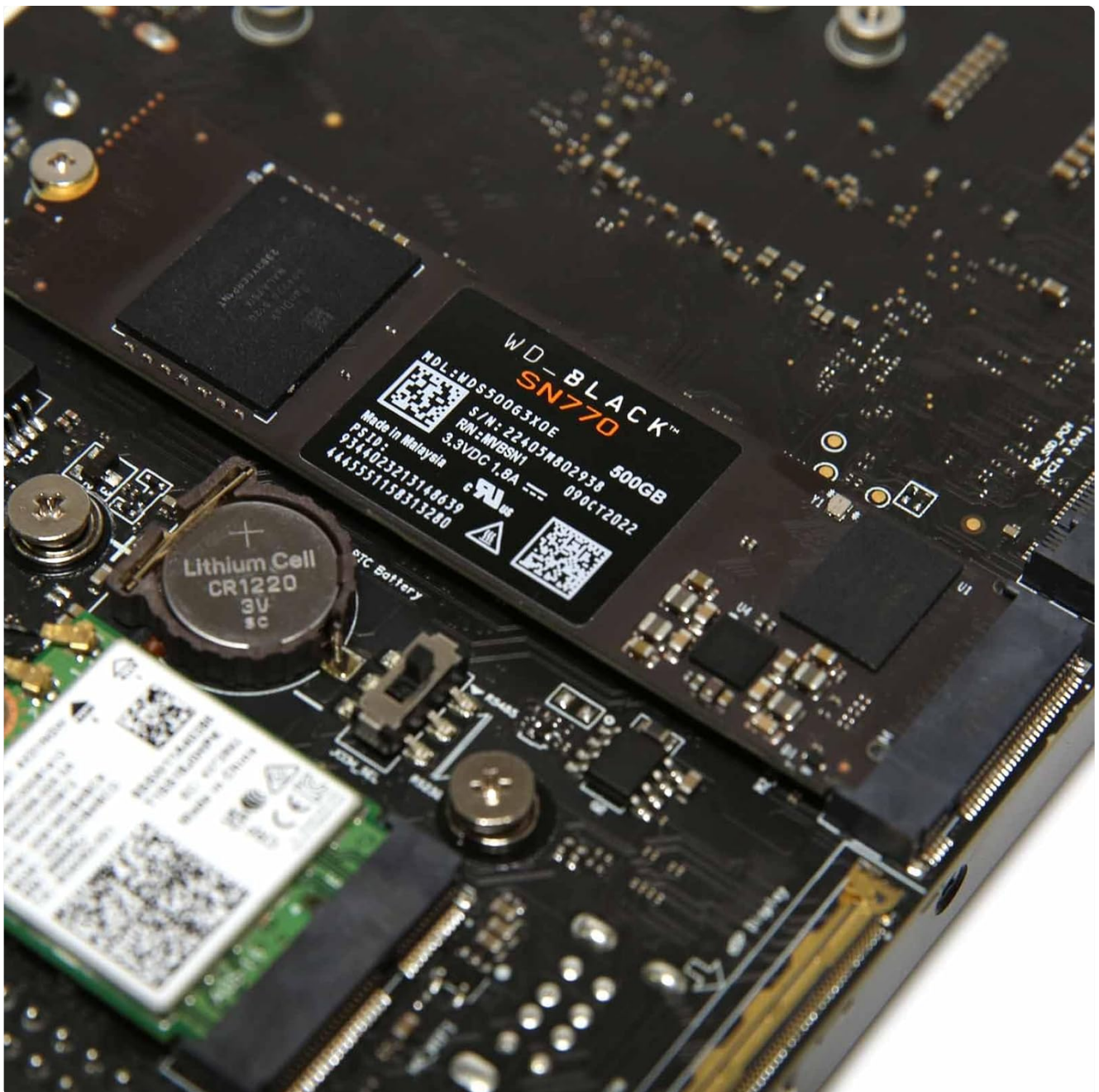
Figure 5: The underside of the board with M.2 slots for SSD and WiFi.
