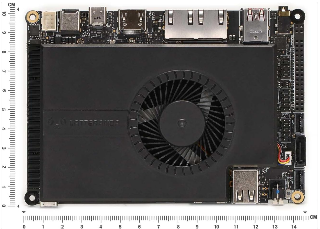
Figure 3: Top view of the LattePanda Sigma, highlighting its compact design.
