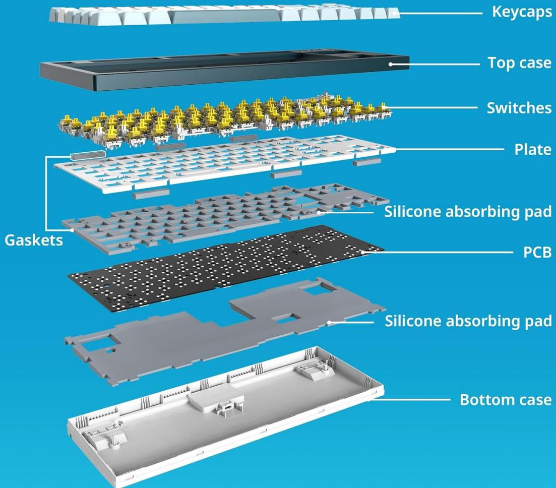
An exploded diagram of the Montech MKey TKL keyboard, detailing its internal structure. Components such as keycaps, top case, switches, plate, gaskets, silicone absorbing pads, PCB, and bottom case are shown separated, highlighting the keyboard's layered design for optimal acoustics and feel.
