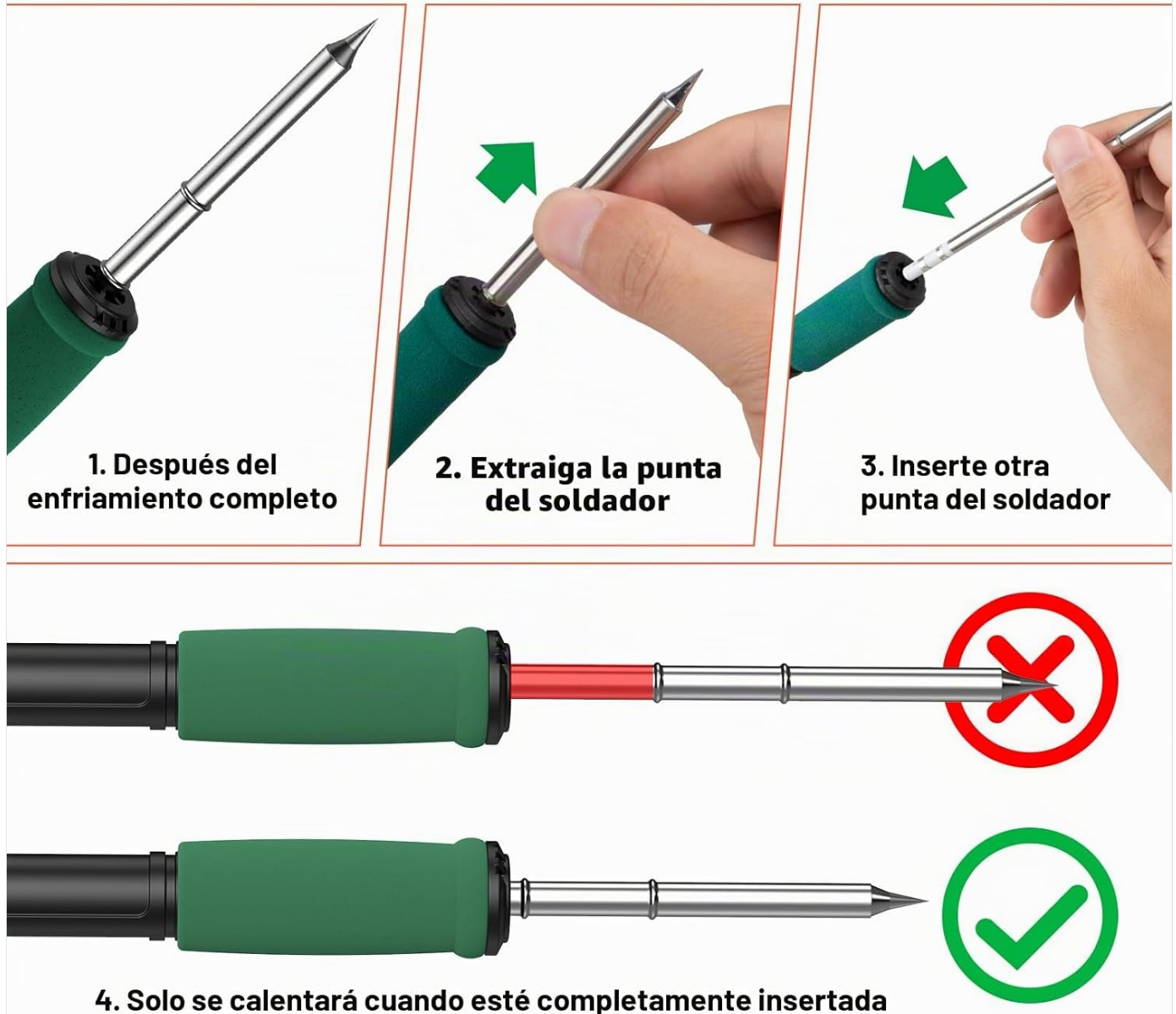
Image 4.1: How to replace the soldering tip. Ensure the tip is fully cooled before removal and fully inserted for operation.
