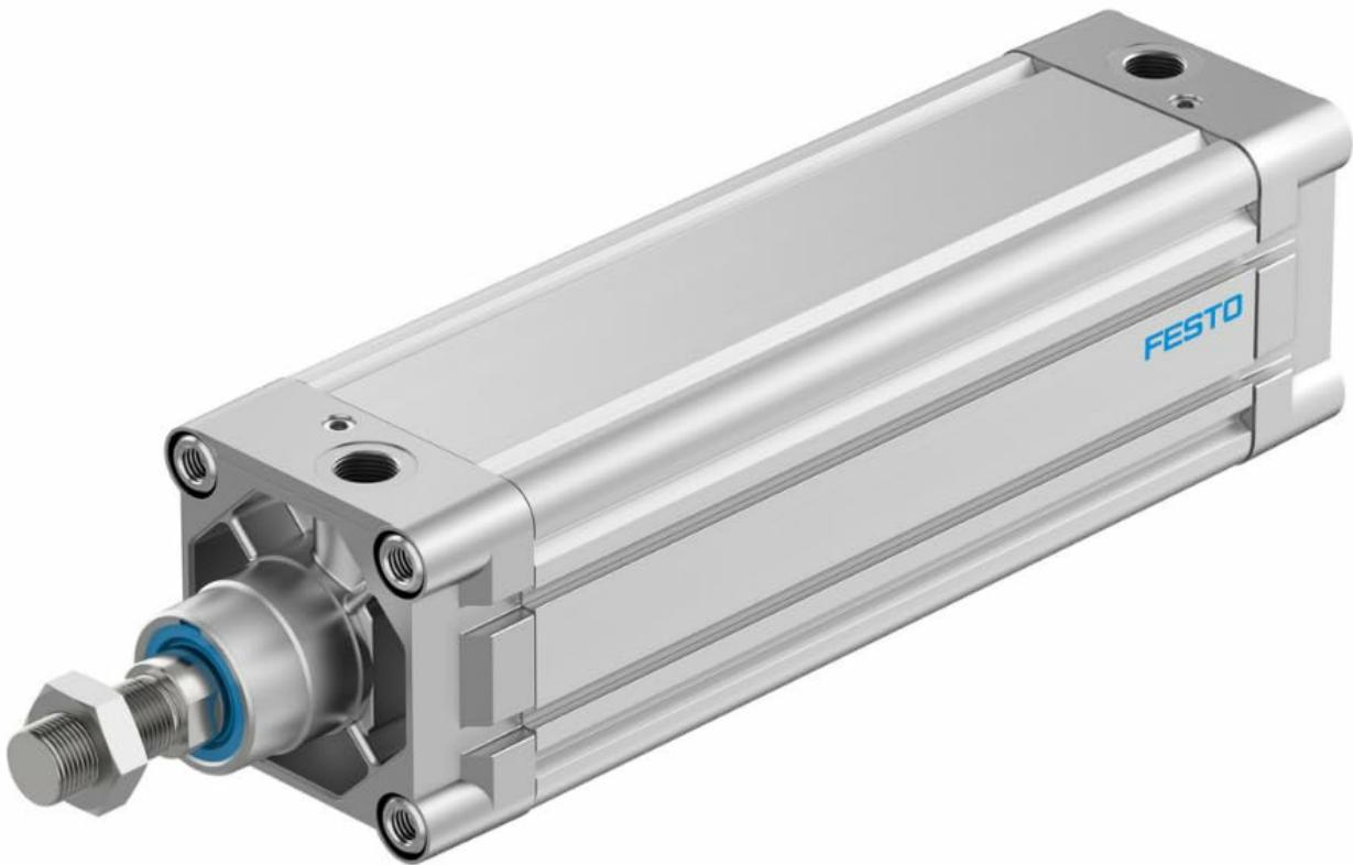
**Figure 1:** FESTO DNC-100-320-PPV-A ISO Cylinder. This image shows the complete pneumatic cylinder assembly, highlighting its profile barrel design, piston rod with external thread, and the integrated pneumatic cushioning at the end caps. The FESTO branding is visible on the side.
