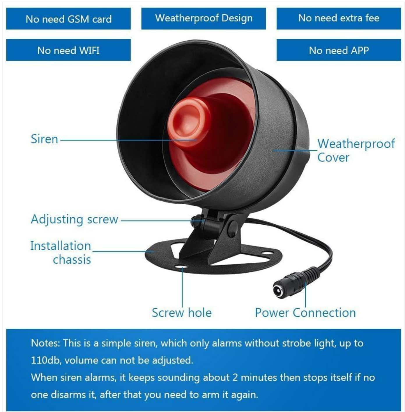
Figure 2: Siren components and installation points.
