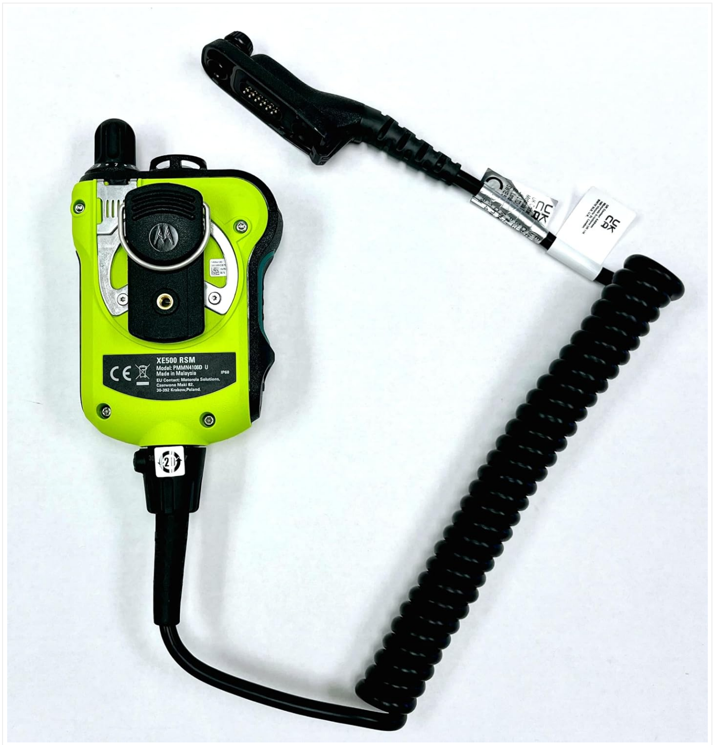
Figure 2: Rear view of the Motorola APX XE500 RSM, showing the integrated cable and the belt clip attachment point. The robust design is evident from this angle.
