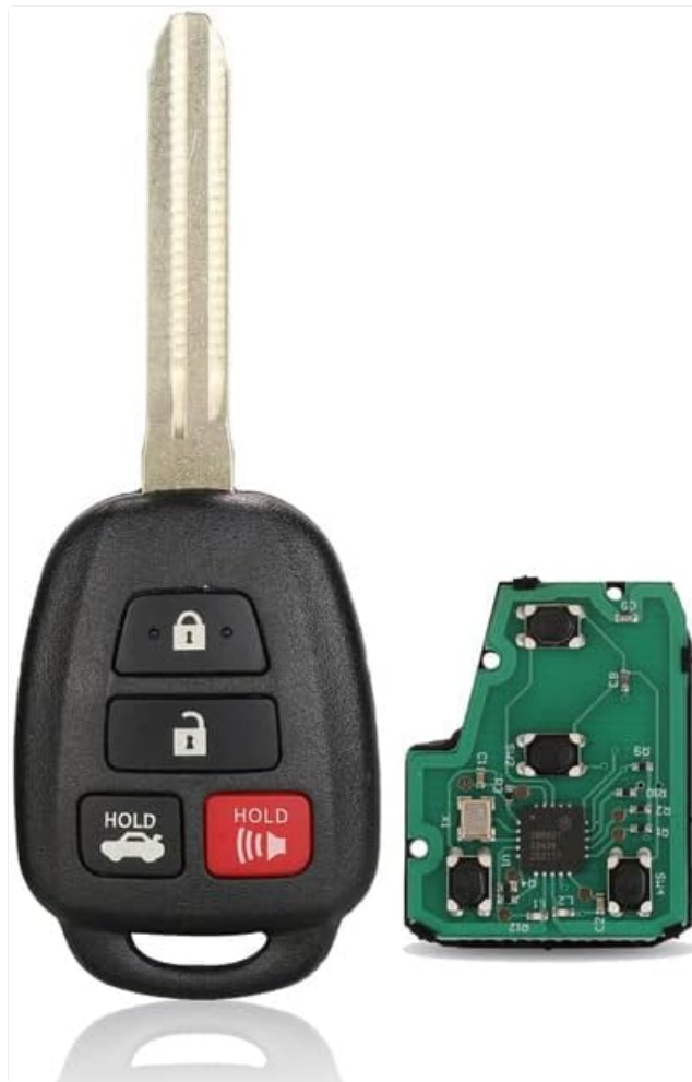
Figure 2.1: This image displays a 4-button remote car key fob alongside its internal circuit board. The key fob features buttons for lock, unlock, trunk release, and a panic alarm. The separate circuit board illustrates the electronic components responsible for the remote functions.
