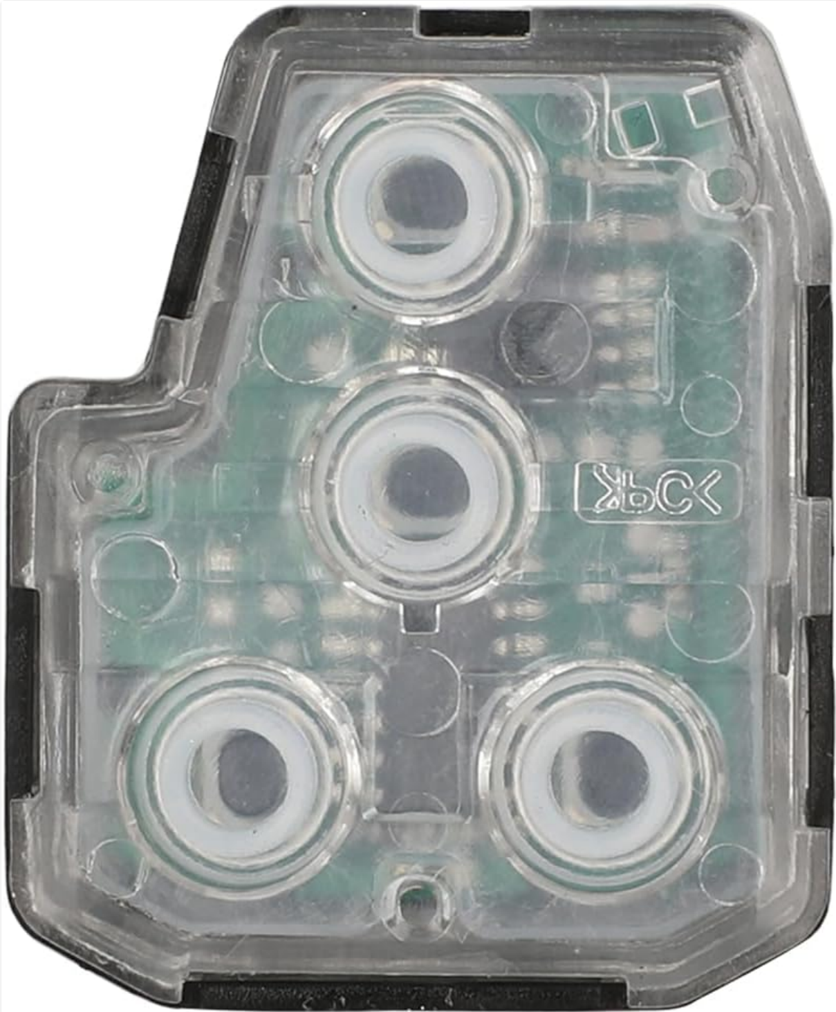
Figure 2.4: A close-up view of the internal rubber button pad, which sits beneath the key fob's outer shell and activates the electronic switches on the circuit board.
