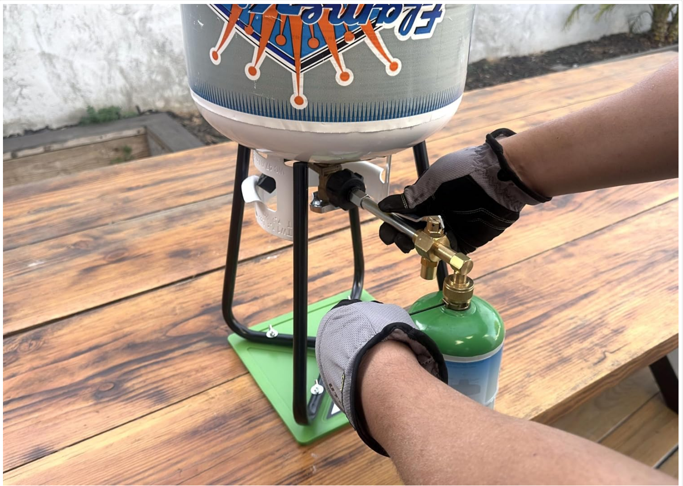
Figure 6: Demonstrating the process of refilling a 1LB propane cylinder from a larger tank using the Flame King refill stand and adapter.
