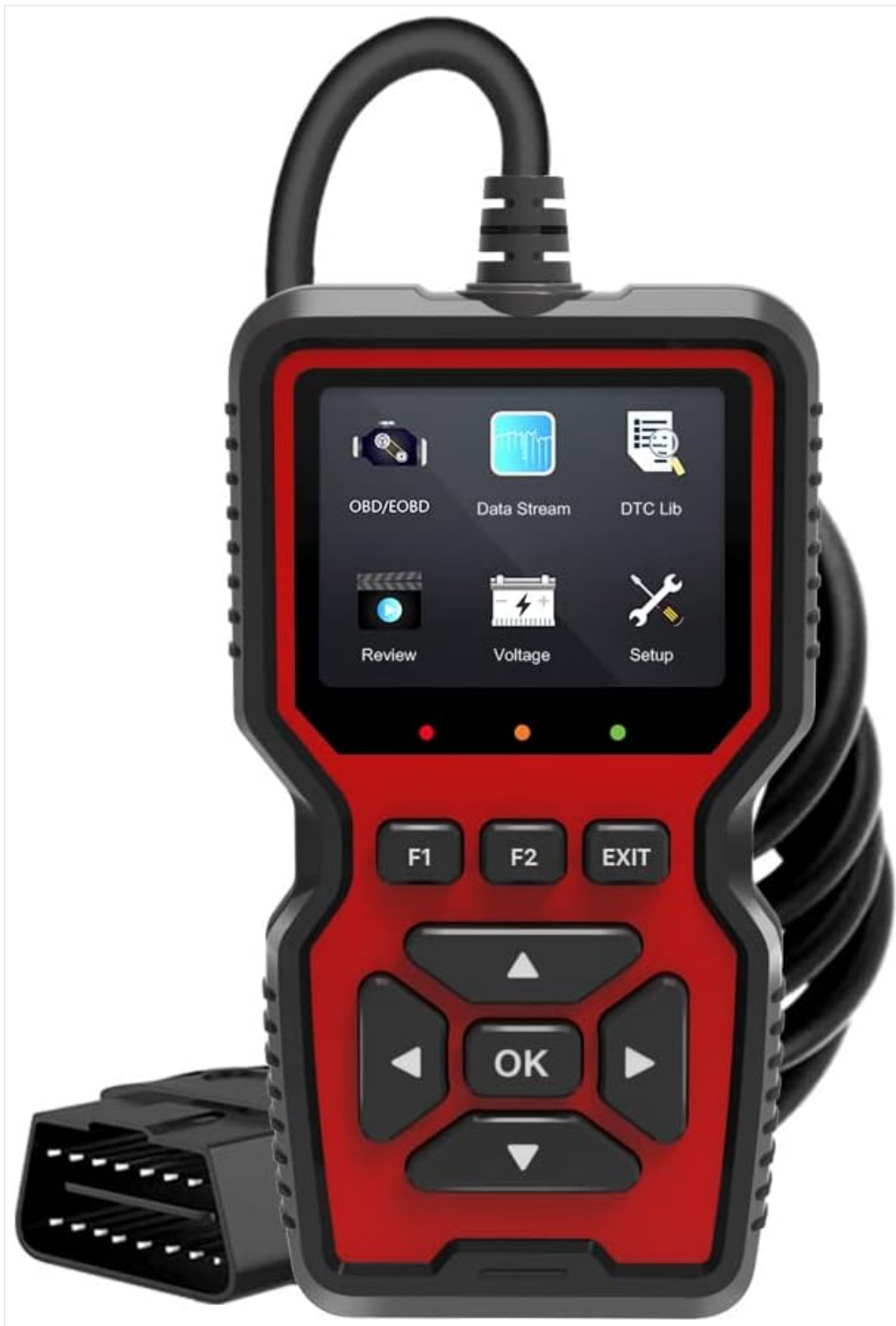
Figure 1: Front view of the Outzone V519 OBD2 Scanner, showing its color screen and control buttons.
