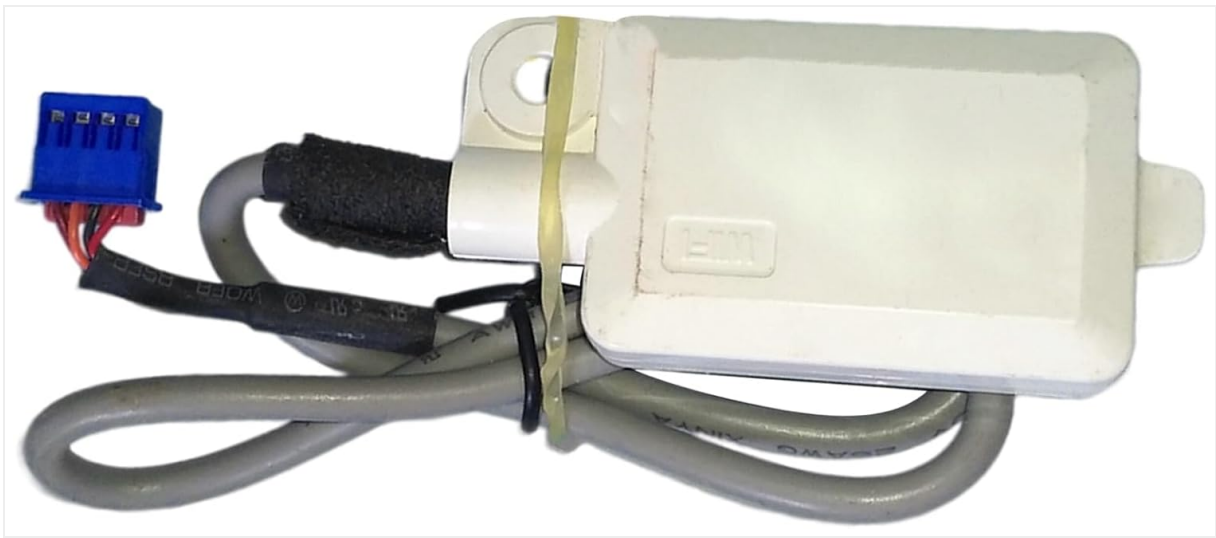
Figure 4.1: A detailed view of the blue multi-pin connector, which is essential for establishing the electrical and data connection between the Wi-Fi module and the Gree air conditioning unit. Observe the specific pin arrangement to ensure correct orientation during installation.
