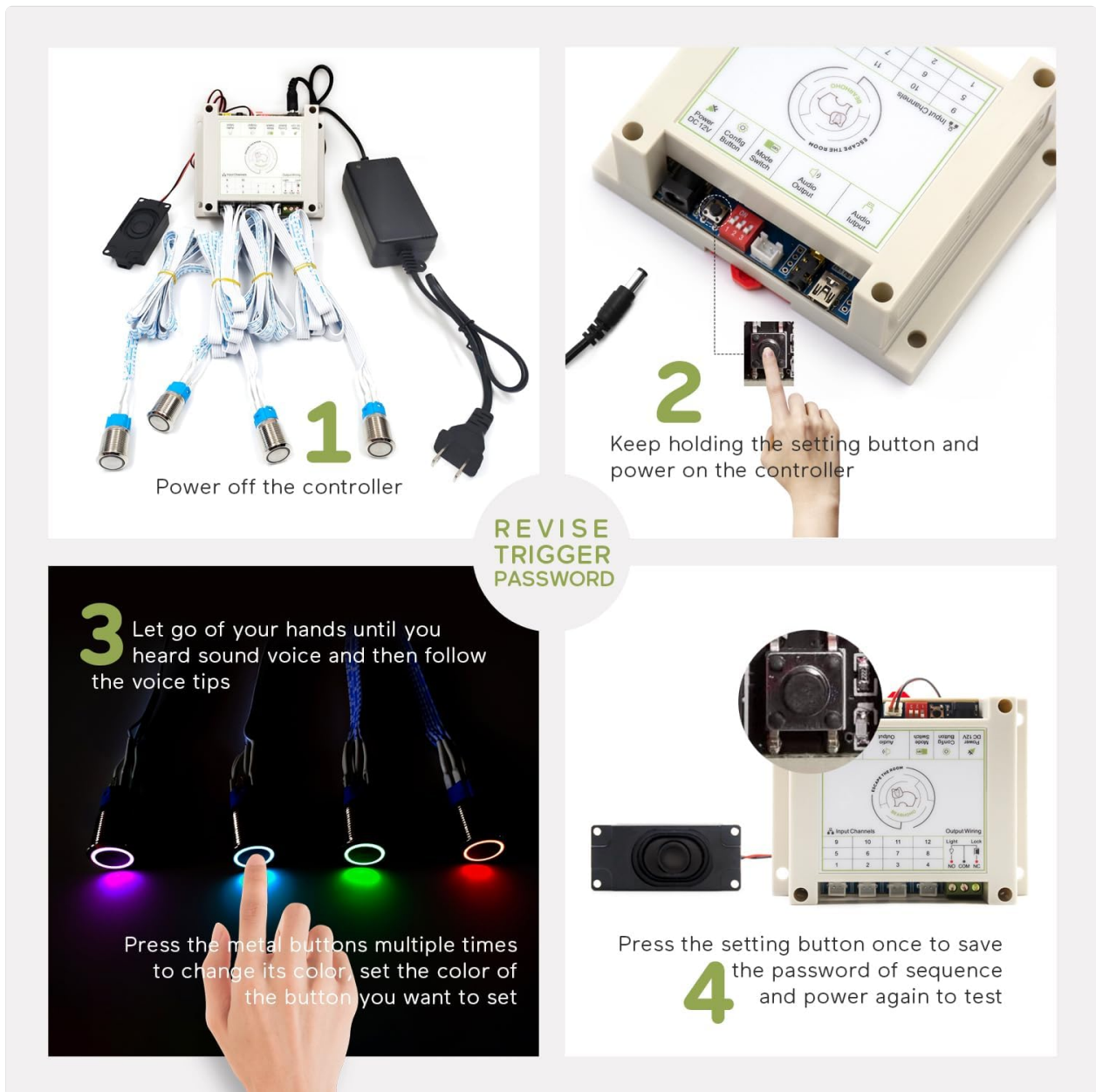
Figure 5: Color Setting Procedure. This image illustrates the steps to modify the required color sequence for the buttons.
