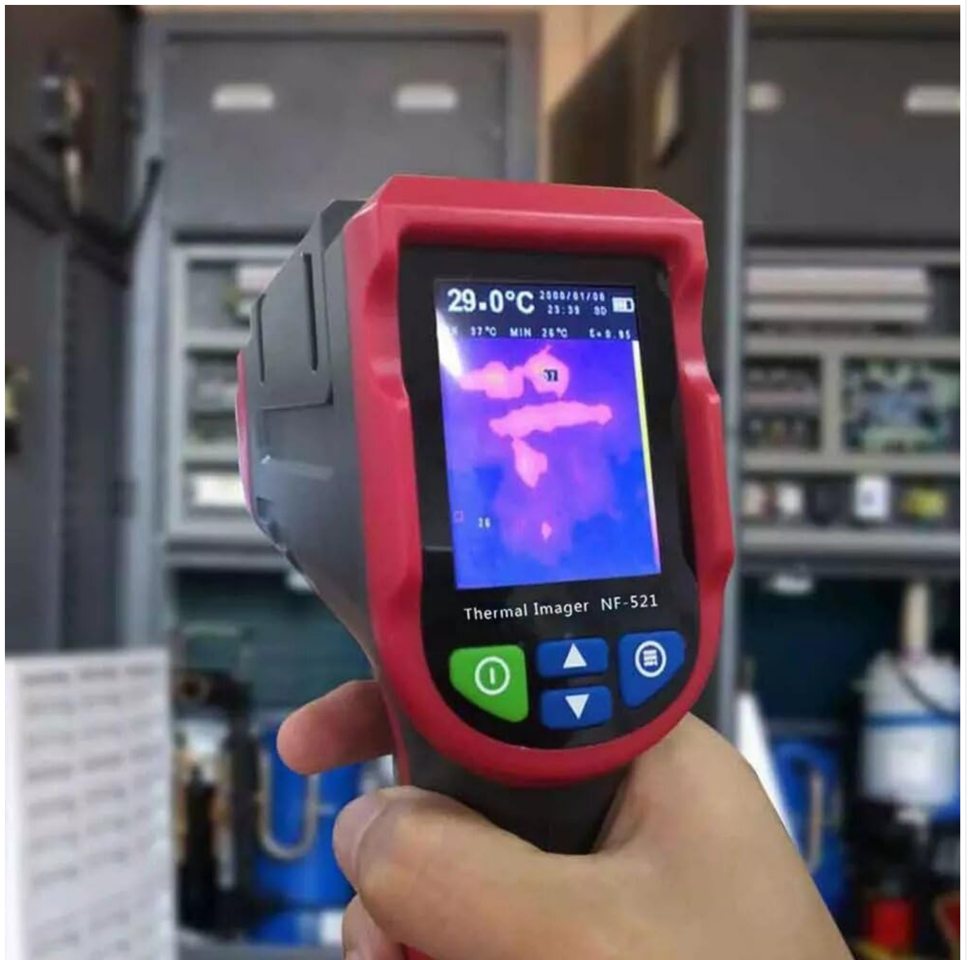
Figure 3: The NF-521 in operation, showing a thermal image on its 2.4-inch screen. The display indicates temperature readings and the thermal distribution of the scanned area.
