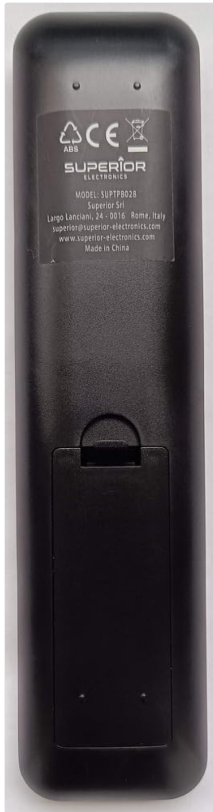
Figure 2.2: Back view of the remote control, displaying the battery cover and the product information label.
