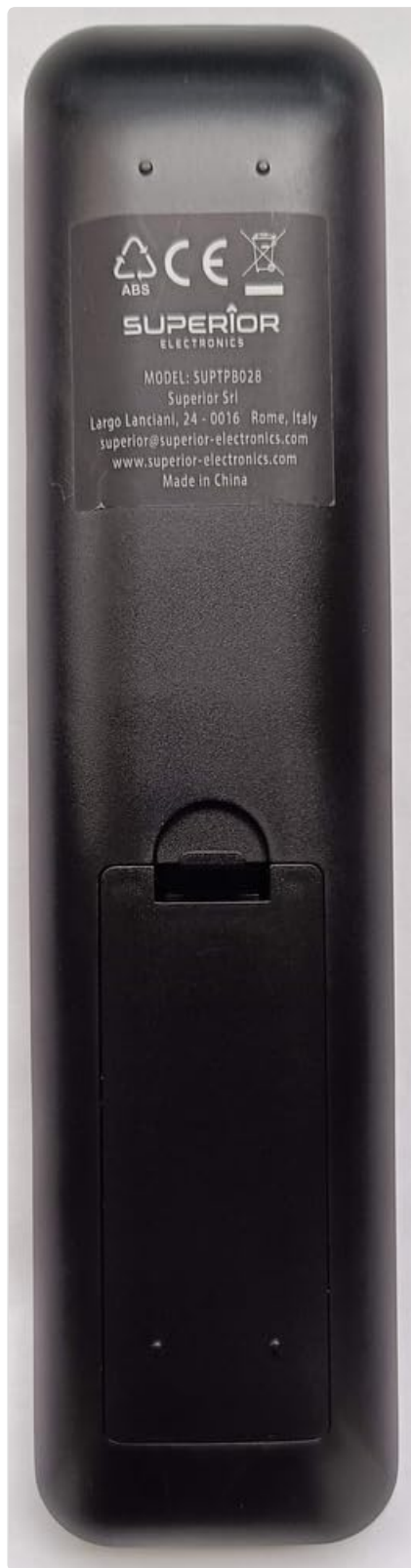
Figure 1: Back view of the remote control showing the battery compartment.
