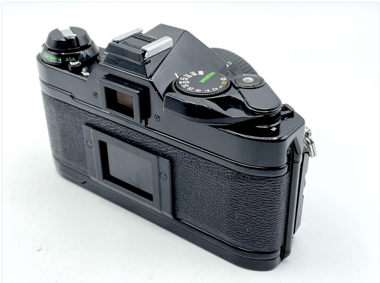
Figure 3.1: Top view of the camera, showing the shutter speed and ISO dials.
