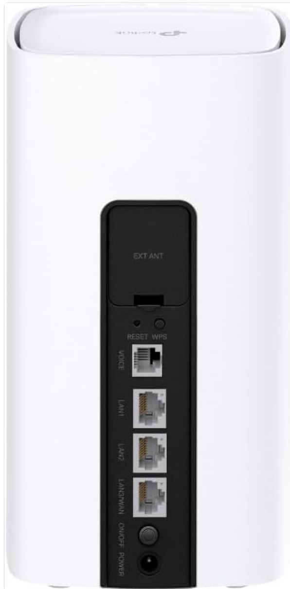
Figure 2.2: Rear view of the TP-Link NX510v router, displaying the various ports including LAN, WAN/LAN, Voice, Reset/WPS, and power input.
