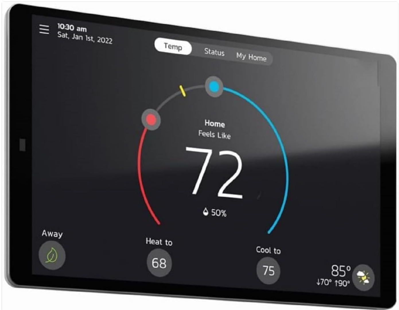
Figure 2: Detailed view of the Lennox S40 Smart Thermostat's main screen with labeled elements for user understanding. This screen is central to operating and monitoring your system.
