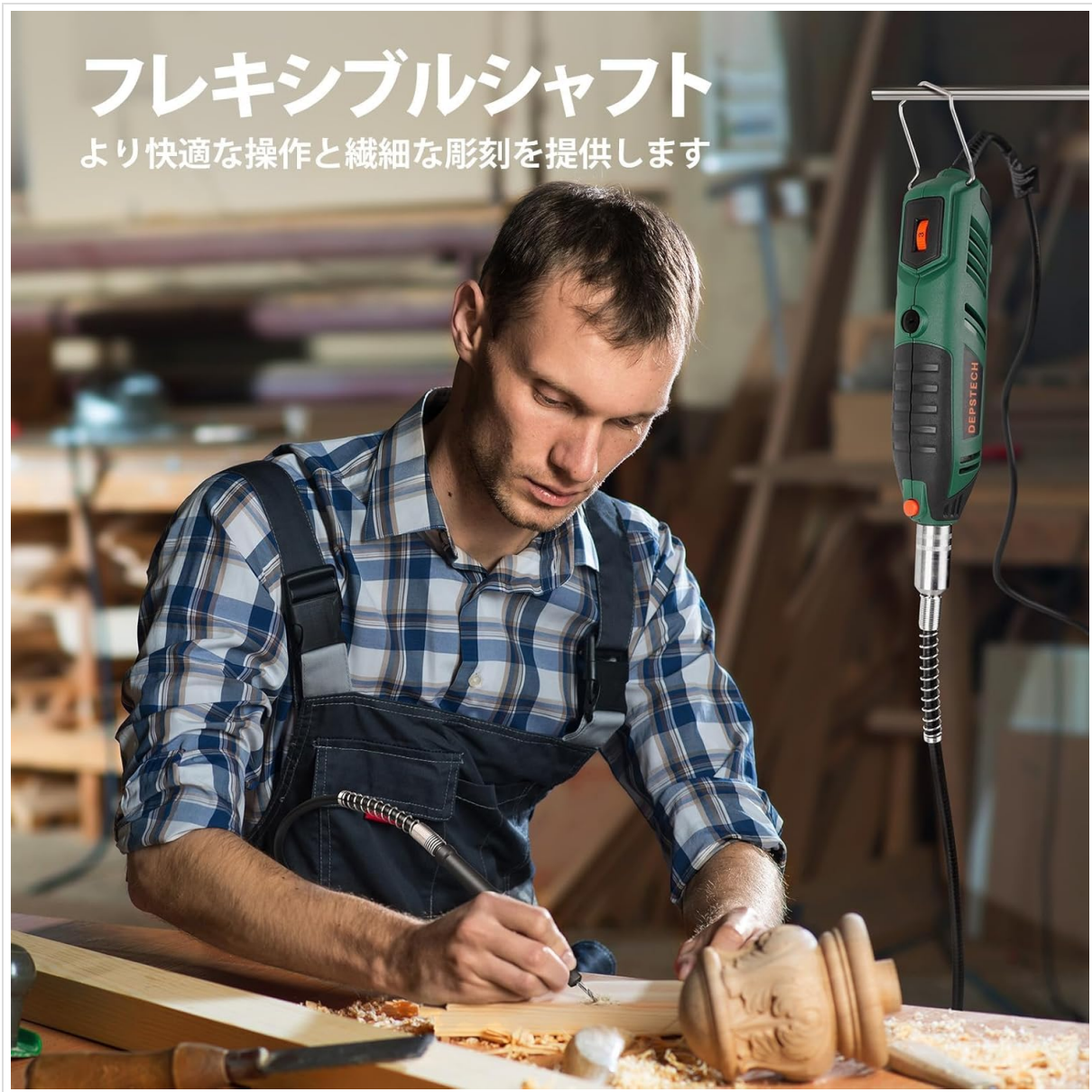
Figure 5: Using the flexible shaft for intricate carving.
