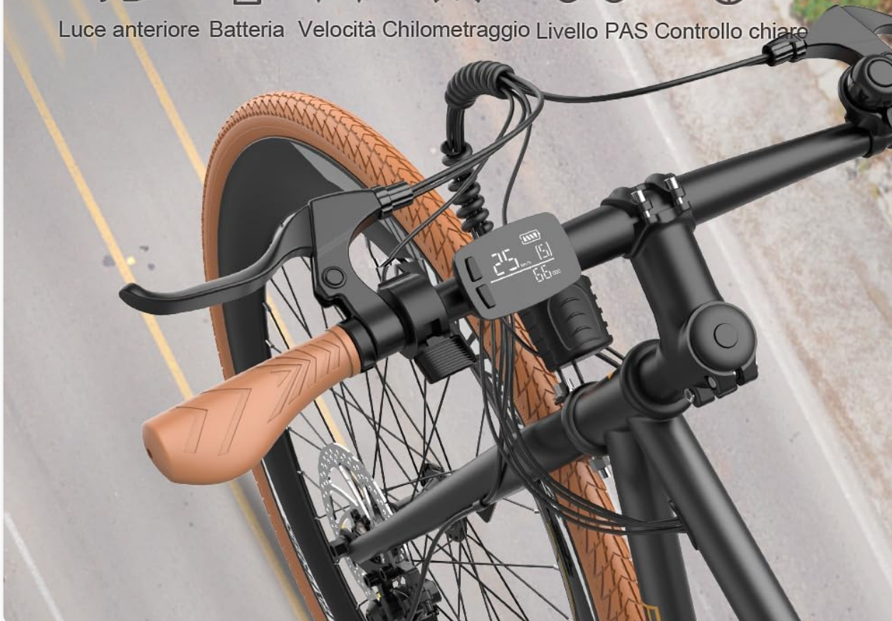
Image 7.1: The LED display showing various riding metrics.
