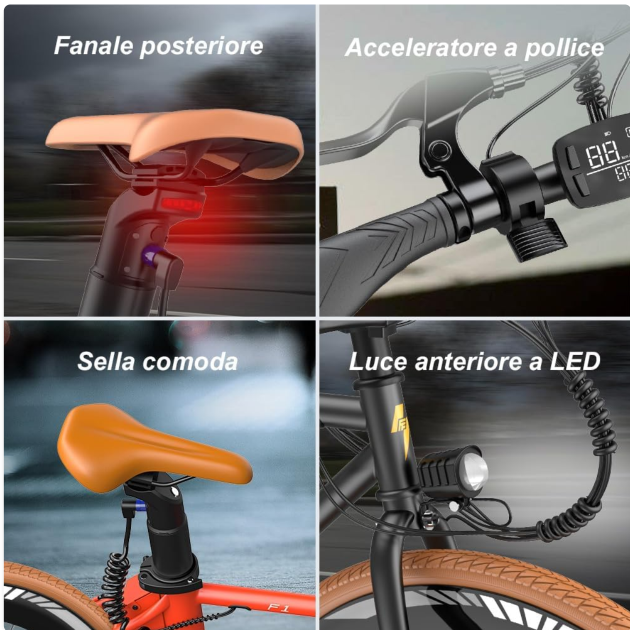
Image 11.1: Key features of the Fafrees F1, including integrated lighting and controls.
